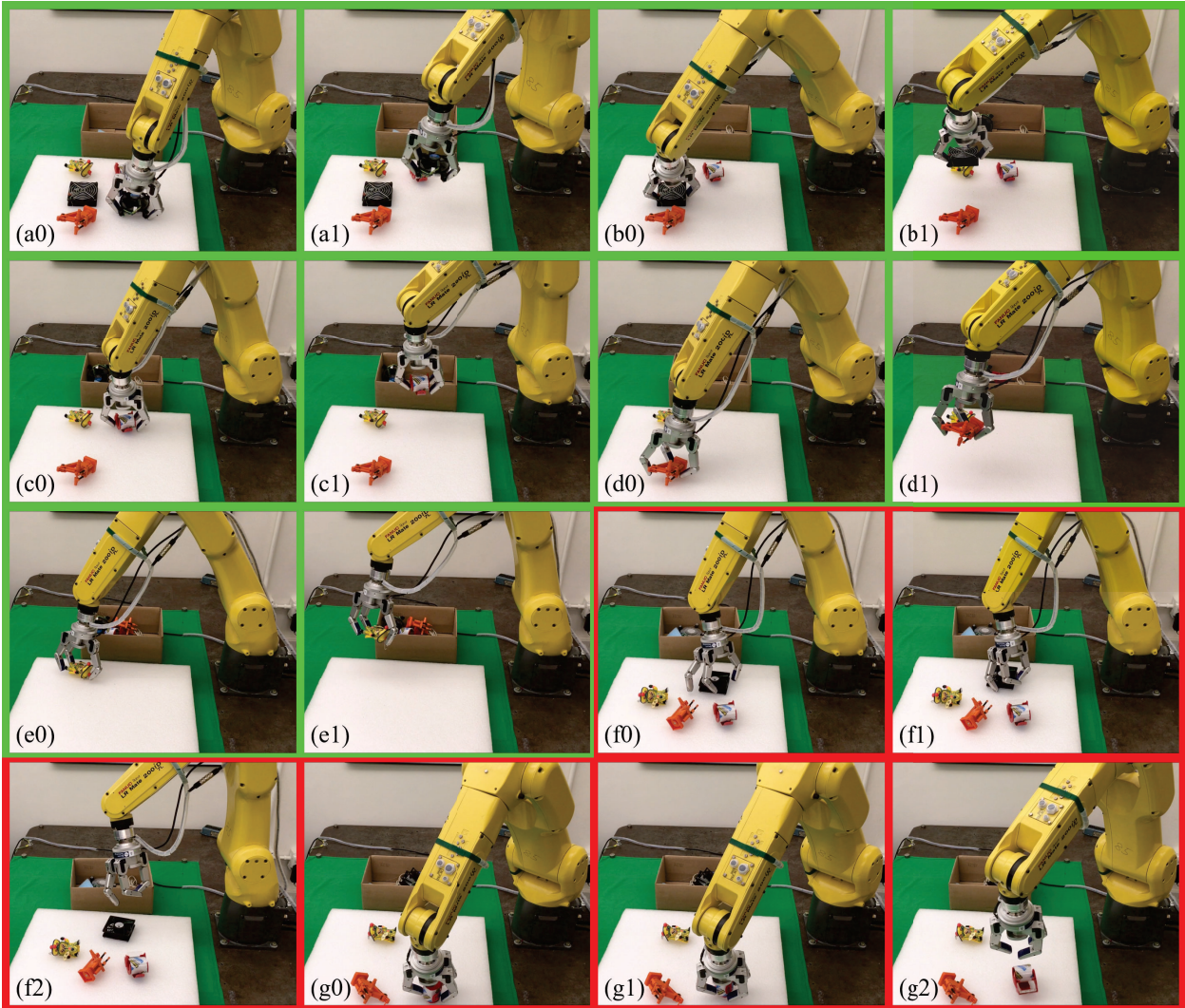
Figure 6.12: Snapshots of grasp planning in clutter environments with success rate 80/97.
