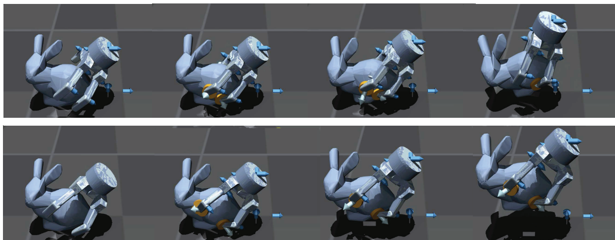
Figure 4.10: Comparison of the initial optimal parallel grasp (Top) and the finger splitting result (Bottom) in a physical simulator.
