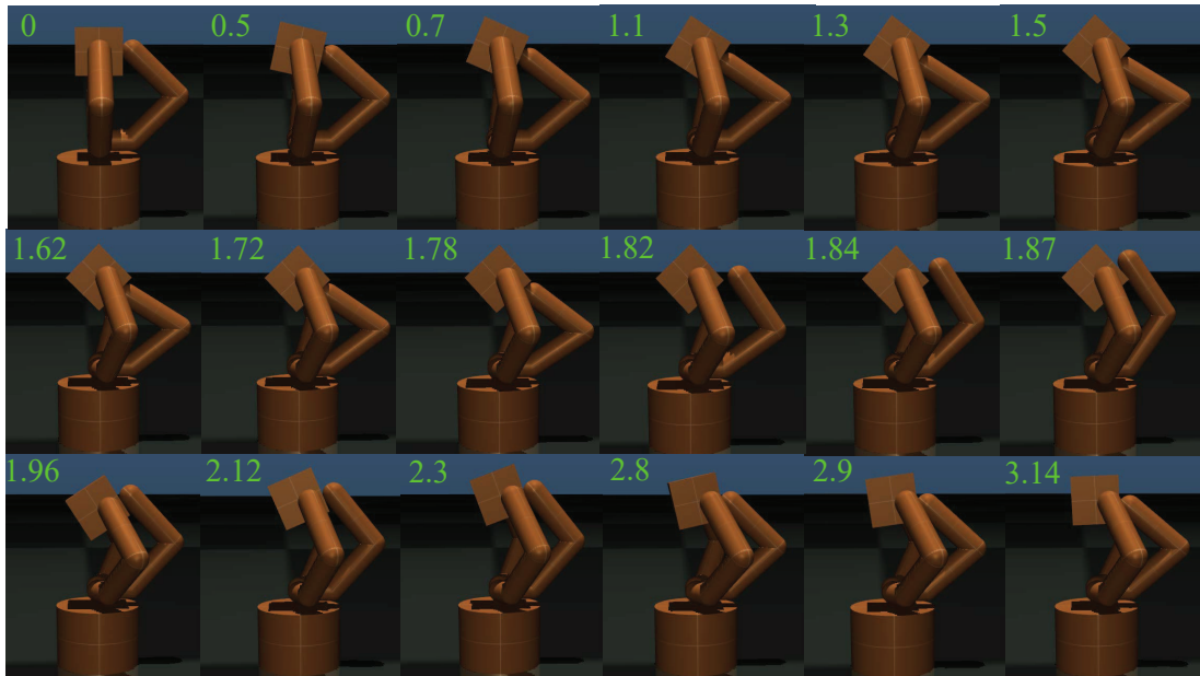
Figure 9.11: Snapshots of box flipping using a three-finger hand.
